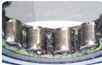
Lubricant degradation caused by electrical discharge currents.
