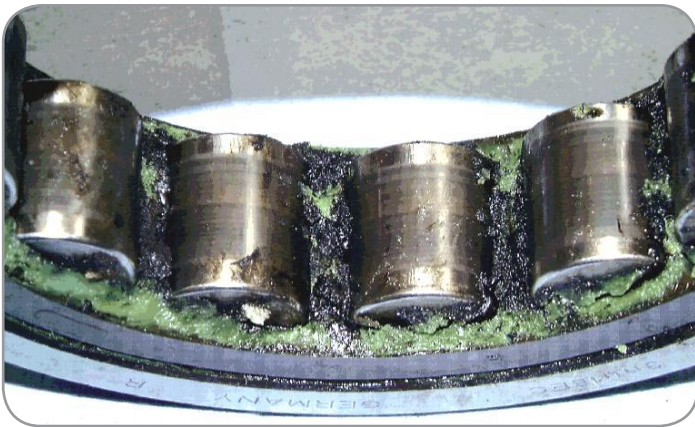
Lubricant degradation caused by electrical discharge currents
