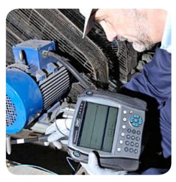
The SKF Microlog Analyzer AX series offers simultaneous triaxial or four-channel vibration measurement capabilities, with fast real-time rate and display updates, all viewed on a vivid 6.4" VGA color display for easy viewing in any light. The result is fast data collection, saving valuable time and money in condition monitoring rounds.
