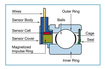
A sensor bearing is composed of:
